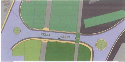
Fig. 11- Possible street redesign implementing traffic circles on either side of the viaducts.
